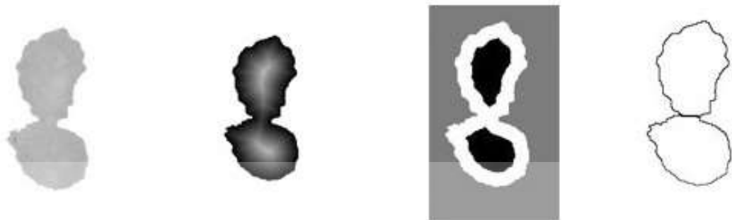
Figure 3.10 Grayscale Image, Euclidean Distance Image, Image After Thresholding, Image After Watershed
