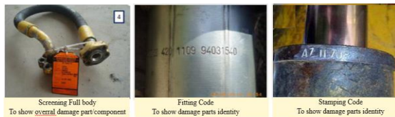
Fig. 12. Documentation of damage part/component
