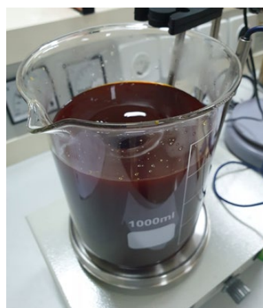
Figure 9. Initial electrolyte mixture during stirring process.
