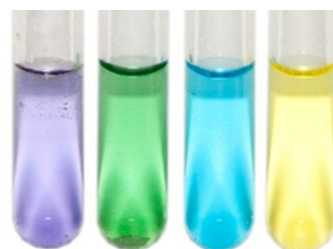
Figure 3. From left: [V(H_2O)_6]^{2+} (Lilac), [V(H_2O)_6]^{3+} (Green), [VO(H_2O)_5]^{2+} (Blue) and [VO(H_2O)_5]^{3+} (Yellow). (Blanc et al., 2010).
