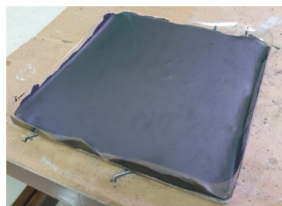
Figure 8. Process of making simple carbon plastic composite on 10 \times 10 \text{ cm} with 1 mm thickness aluminum metal plate.
