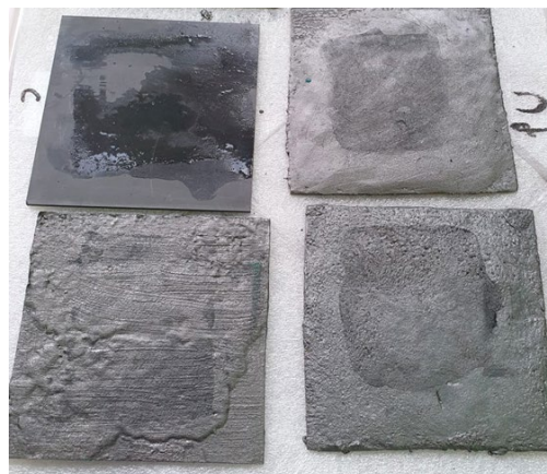
Figure 12. Corrosion problems for all simple carbon plastic composites.
