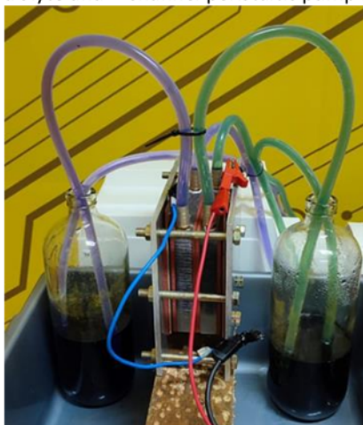
Figure 4: Single cell 10x10cm size Vanadium redox flow battery prototype.
