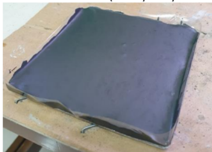
Figure 8: Process of making simple carbon plastic composite on 10x10 cm with 1 mm thickness aluminum metal plate.
