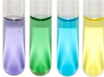
Figure 3: From left: [V(H_2O)_6]^{2+} (Lilac), [V(H_2O)_6]^{3+} (Green), [VO(H_2O)_5]^{2+} (Blue) and [VO(H_2O)_5]^{3+} (Yellow). [6].
