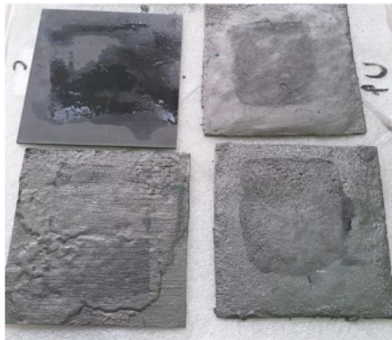
Figure 14: Corrosion problem for all simple carbon plastic composites.
