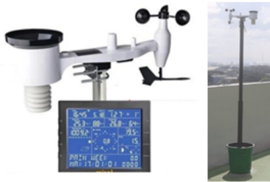
Figure 3: Weather Station Consists of Outdoor Sensors and Indoor Monitor. Outdoor Sensors Are Supported By 2-Meter Pole with Cemented Bucket.
