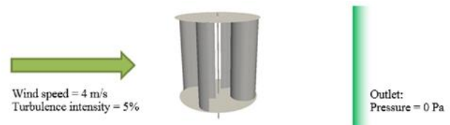
Figure 7: Simulation boundary conditions for turbine CFD analysis.
