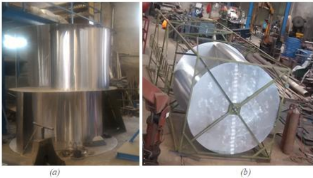
Figure 17: Prototype constructions for both (a) Two-Level and (b) One-Level wind turbines.
