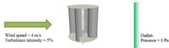
Figure 7: Simulation boundary conditions for turbine CFD analysis.
