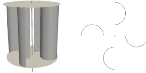
Figure 6: Baseline design for one-level Savonius wind turbine and cut-section of the blades.
