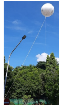
Figure 6: Air Balloon With 3 Anchoring Ropes for Position Stability. Weather Station Outdoor Sensors Are Hung to The Air Balloon.
