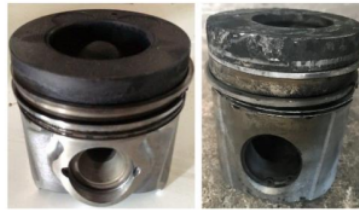
Fig. 4. Original and piston in the transport utility vehicle engine
