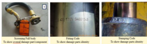
Fig. 12. Documentation of damage part/component
