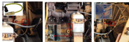
Fig. 10. Temperature, level, and speed sensor location.
