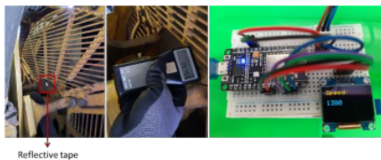
Fig. 7. Fan speed sensor working test.
