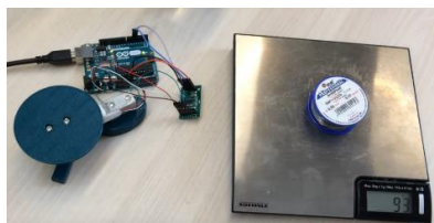
Fig. 6. Load cell sensor working test
