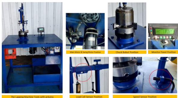
Fig. 10. Lapping machine tools with arduino
