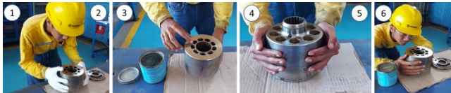
Fig. 2. Manual Lapping by Mechanic
