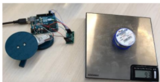
Fig. 6. Load cell sensor working test
