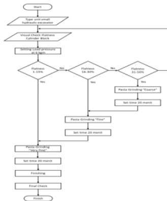
Fig. 5. Tools lapping machine flow diagram.
