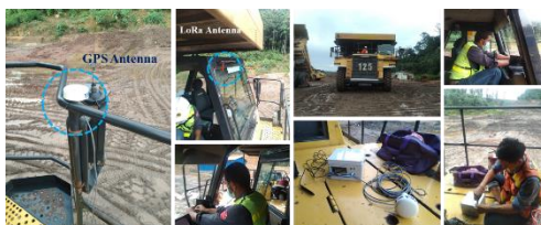
Fig. 15. Installation process in dump truck HD785-7
