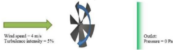
Figure 6. Simulation boundary conditions for turbine CFD analysis.
