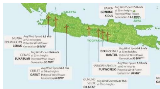
Figure 1. Wind energy potential in several areas in Java, Indonesia (Badan Pengkajian dan Penerapan Teknologi (BPPT), 2014)
