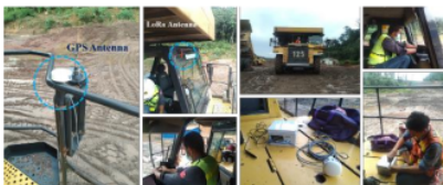
Fig. 15. Installation process in dump truck HD785-7
