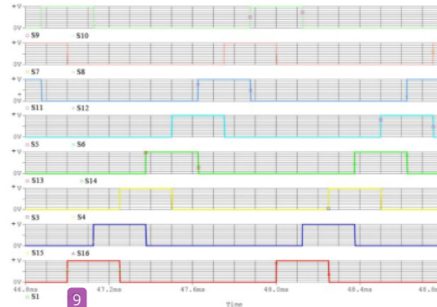
Fig. 12. The switching state of the proposed MV AC-DC converter architecture with 8-channel configuration and a phase shift 45^\circ
