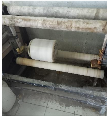
Figure 10. Ceramic suspension mixing using Pot Mill
