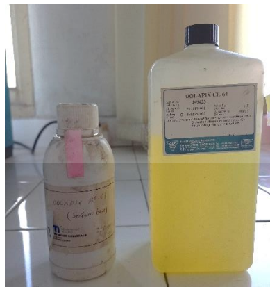
Figure 9. Dolapix PC67 (Left) and Dolapix CE64 (Right) as the Deflocculant
