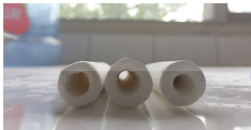
Figure 17. Alumina-Kaolin Membrane Produced using Dolapix CE64 in different Slip Casting Time (3 minutes, 5 minutes and 6 minutes)
