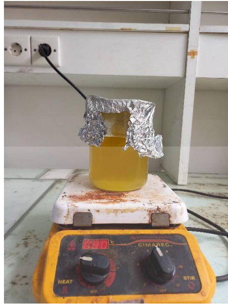
Figure 3. Mixing of Biodiesel and Glycerol-Water using Magnetic Stirrer
