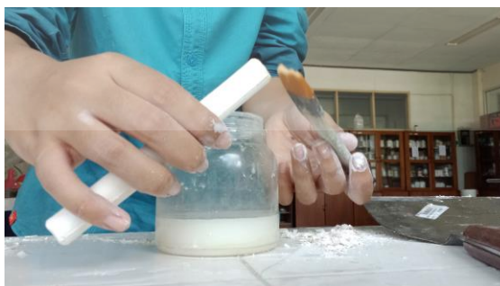
Figure 13. Finishing of the Casted Membrane before Drying in Oven
