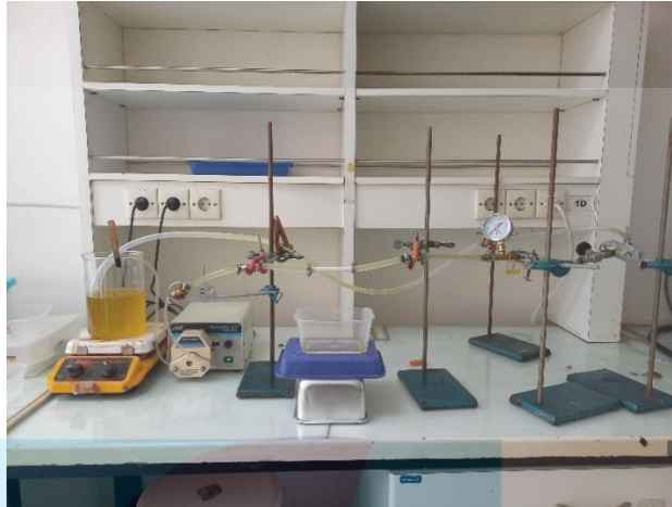
Figure 1. Microfiltration Experiment with Feed of Biodiesel-Glycerol mixture
