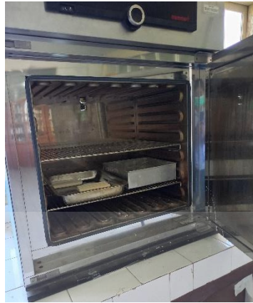
Figure 14. Drying the Casted Membrane in the Oven
