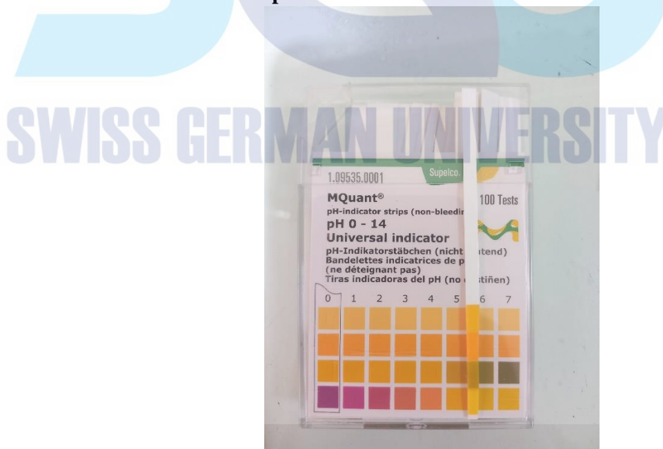
Figure 6. pH test for the Buffer Solution using Universal Indicator shows the value between 5.0-6.0
