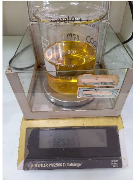
Figure 5. Weighing Biodiesel for Feed Mixture Preparations
