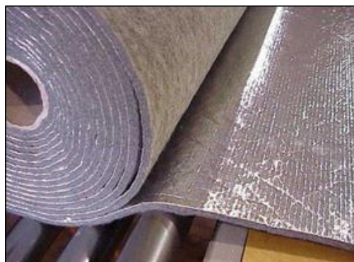
Figure 22. Aluminium thermal insulation
