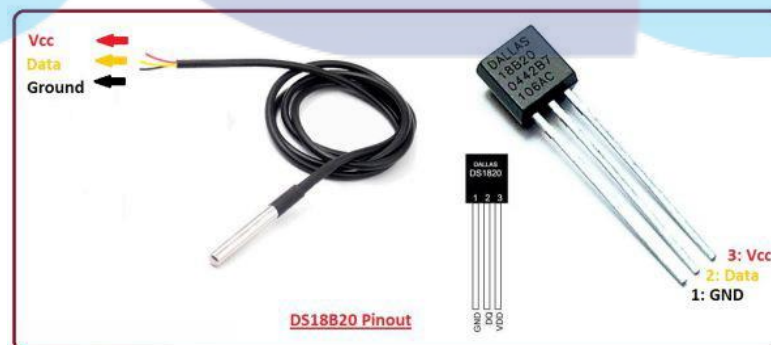
Figure 14. DS18B20 Temperature Sensor pin layout
