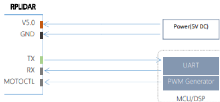
Figure 3-3 RPLIDAR A2 Pins Reference Design
