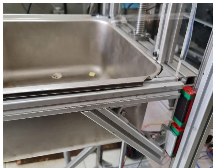
Figure 7. Added Framework on the Sink Holder
