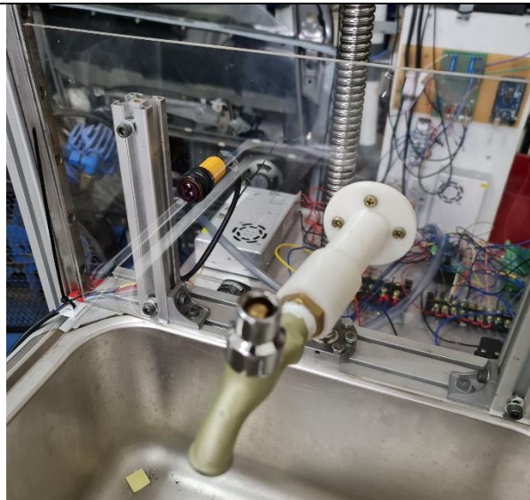
Figure 11. 2nd Infrared Sensor for Automatic Hand Wash Cycle Switch
