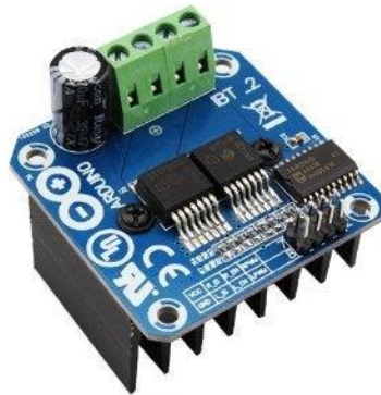
Figure 25. Motor Driver IBT-2
