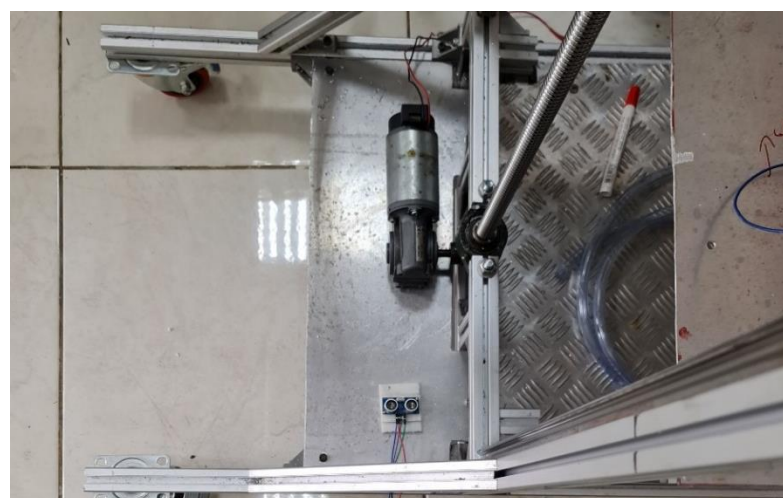
Figure 9. 2nd Ultrasonic Sensor for Sink Height
