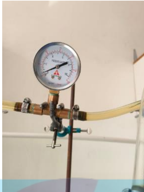
Figure 3. Microfiltration Experiment Pressure Gauge at 0.5 \text{ kg/cm}^2
