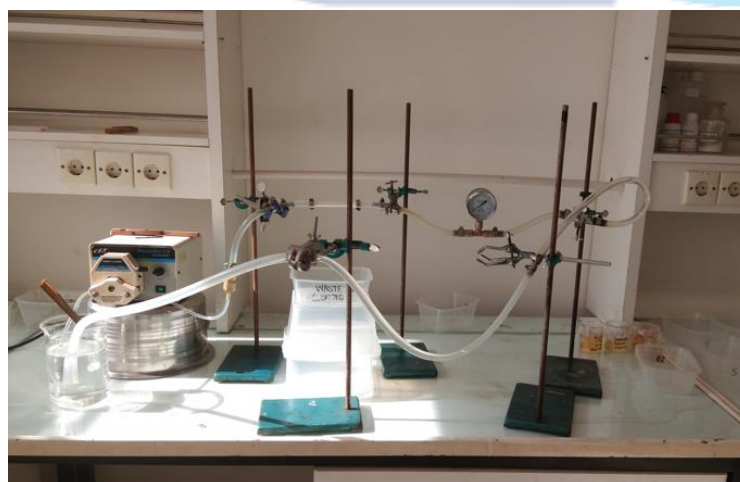
Figure 2. Membrane Cleaning after Microfiltration Experiment
