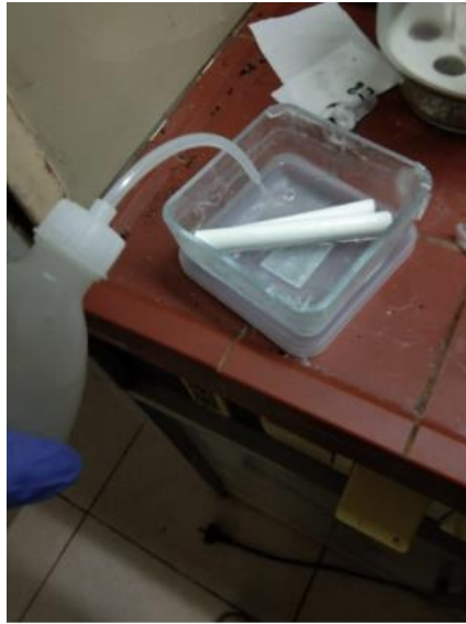
Figure 6. Rinsing the Ceramic Membranes with Ethyl Acetate after immersing
