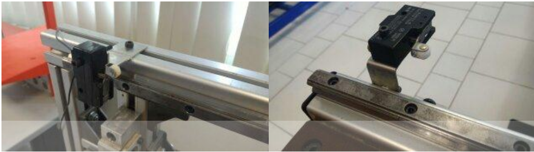
Figure 3-17 Limit switch installed to the table
